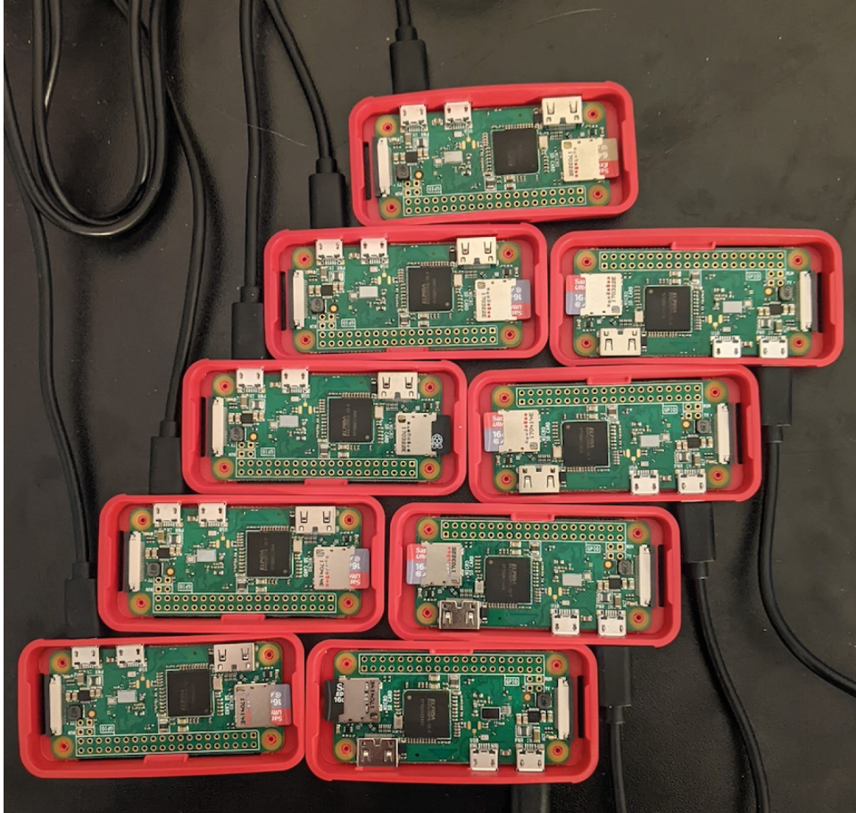
Fig. 4. 9 Raspberry Pi Zero W devices loaded with the LOADHoC Prototype
